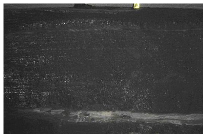
Figure 2 - Photo taken of an underground longwall face which shows characteristic darker coal and lighter marker band features. A dominant marker band is seen at the bottom of the image, as well as finer, less immediately obvious bands above. The top of the image shows sections of the roof canopy support.
