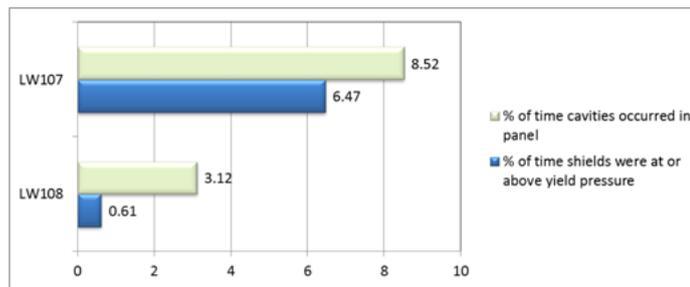
**Figure 6 - Shield effectiveness determined from LVA data**
