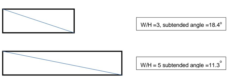
Figure 5 - Kinematically acceptable mechanism for pillar collapse
