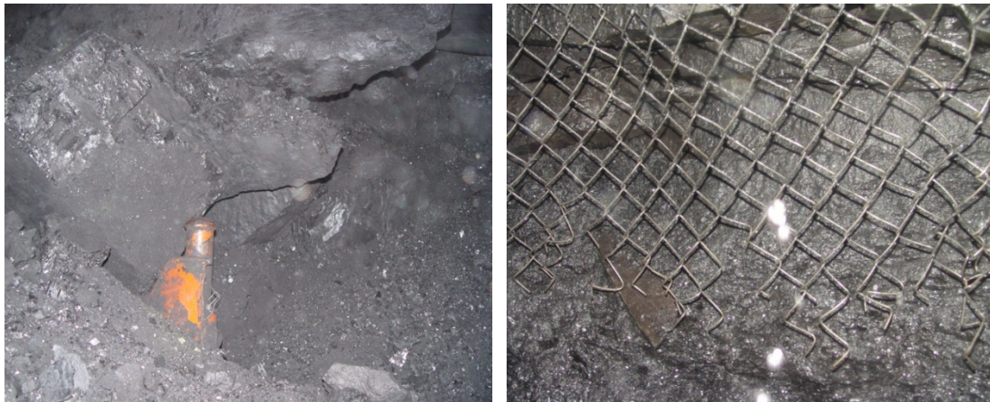
Figure 1 - Normal coal from Sihe outburst site (left) and tectonically disturbed coal from outburst cavity at Menin Mine, Henan, China (right)
