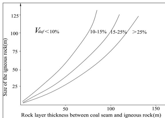
Figure 7 - Variation curves of  $V_{daf}$  with rock bed thickness and distance between rock bed and coal seam in certain coal mine
