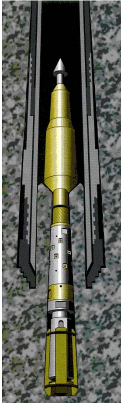
Figure 1 - Pictorial view of overcoring operation Figure 2 - Example of diameter change with time during overcoring
