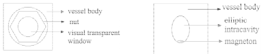
Figure 3 - Frontal view of the view cell Figure 4 - Cross section of the view cell
