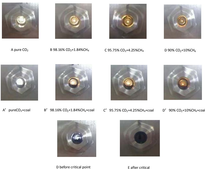
Figure 6 - Pictures of critical points of different components of the CO 2 -CH 4 binary system and CO 2 -CH 4 +coal system
