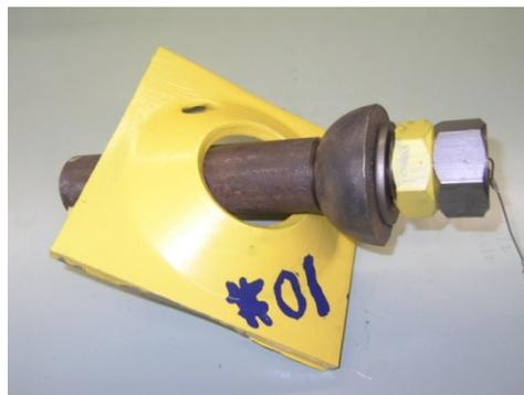
Figure 6 - Typical load cell mounted on a rebar
