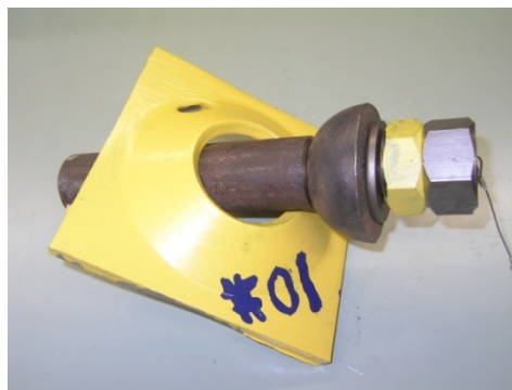
Figure 6 - Typical load cell mounted on a rebar
