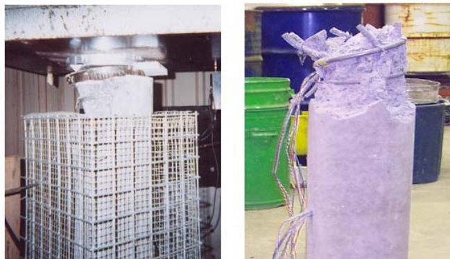
Figure 2 - Failure of the internally reinforced concrete column
