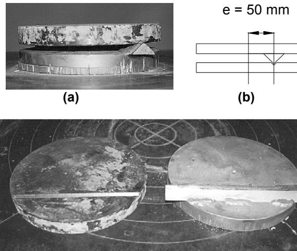
Figure 1 - Steel end plates for eccentric loading
