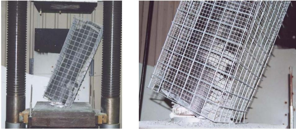
**Figure 3 - Failure of the carbon fibres column**
