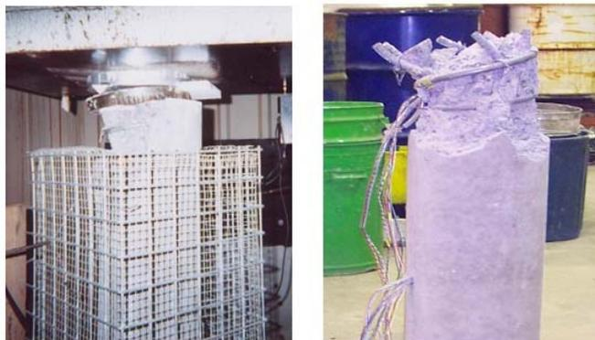
**Figure 2 - Failure of the internally reinforced concrete column**
