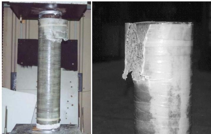
**Figure 4 - Failure of the E-glass wrapped column**
