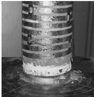
Figure 6 - Failure of the steel strapped column with 10 mm spacing
