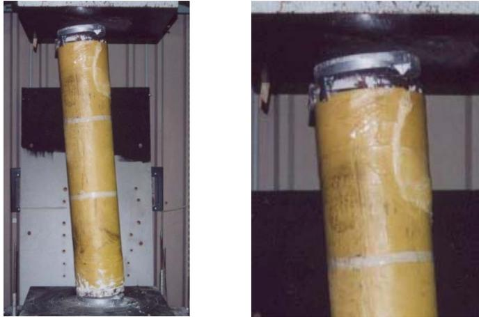
**Figure 5 - Failure of the Kevlar wrapped column**
