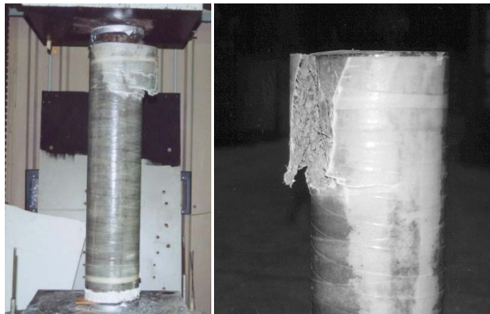
Figure 4 - Failure of the E-glass wrapped column
