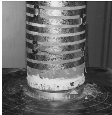
**Figure 6 - Failure of the steel strapped column with 10 mm spacing**
