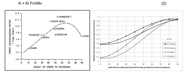
Figure 12 - Concentration of horizontal stresses at the maingate corner (a:-principal stress, b: stress factor for component normal to roadway centreline - Fm)
