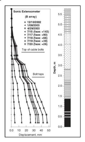
Figure 1 - Vertical movements above a 4.9 m wide roadway showing a height of fracturing of 4.9 m above a 4.9 m wide roadway (from Mark, et al., 2007)
