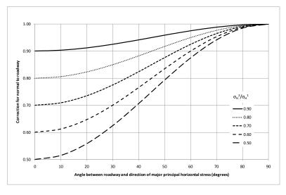
Figure 10 - Stress factor for roadway alignment (Fa)
