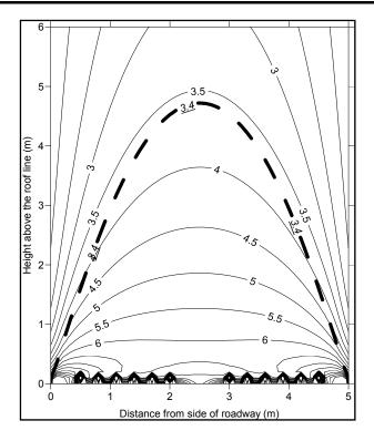
Figure 4 - Extent of failure zones above a 5 m by 2.5 m roadway for different CI values (thin lines) and for a spalling limit of 3.4 (heavy dashes) for K=1.3 and E/G=15
