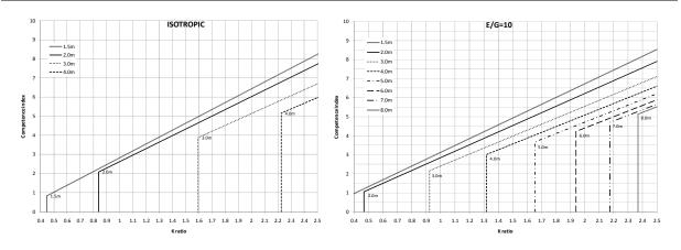
Figure 6 - The height of failure above a 5 m by 2.5 m roadway as a function of the K ratio and the competence index (a: Isotropic, b: E/G=10)
