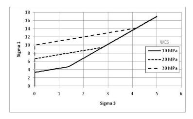
Figure 3 - Adopted failure criterion for coal measure rocks
