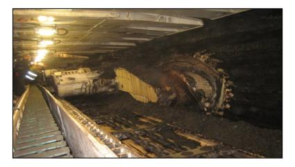
Figure 3- Double drum shearer and shield support in East 1
