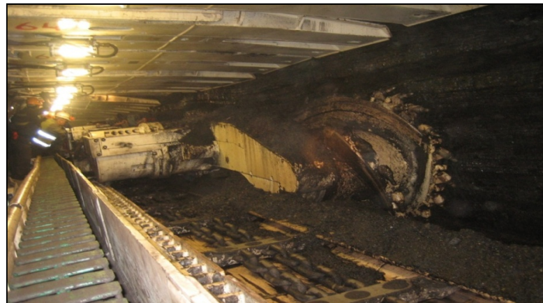
Figure 3- Double drum shearer and shield support in East 1
