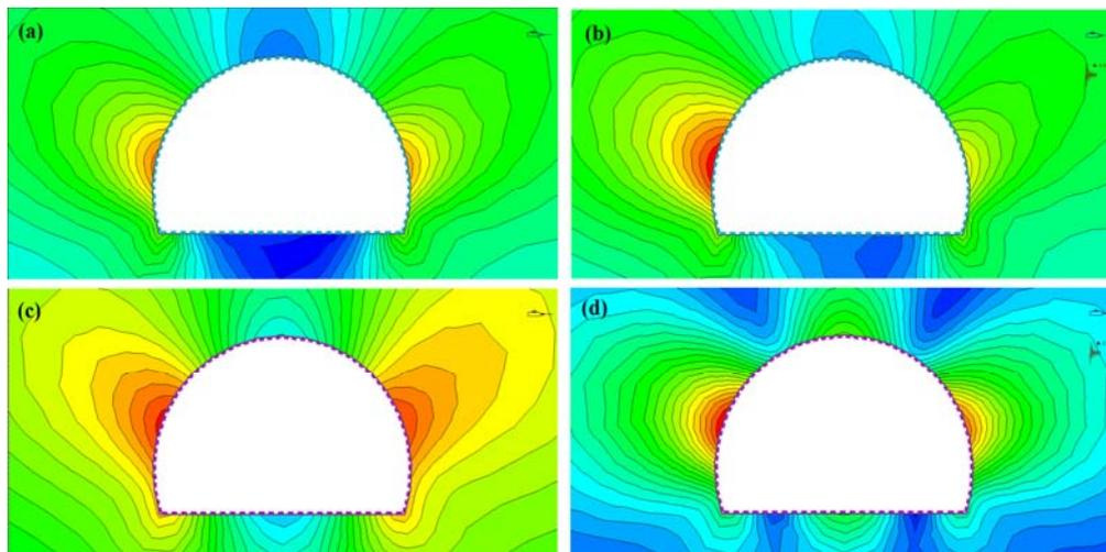
**Figure 5 - The displacement with support system, a) shotcrete with 5 cm thickness, static, b) shotcrete 5 cm with thickness, dynamic c) shotcrete with 15 cm thickness, static, d) shotcrete 15 cm with thickness, dynamic**
