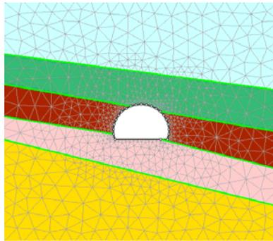
Figure 1 - The tunnel modelled by Phase2 software
