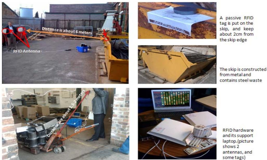
**Figure 6 - Communication range testing for passive RFID equipment.**
