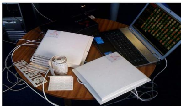
**Figure 5 - Passive RFID equipment with corresponding antennas**
