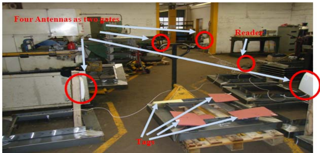
Figure 8 - Scenario for testing two gates or 'choke points' in the factory
