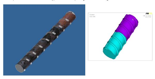
Figure 1 - Model of a steel bolt showing a typical rib profile.
