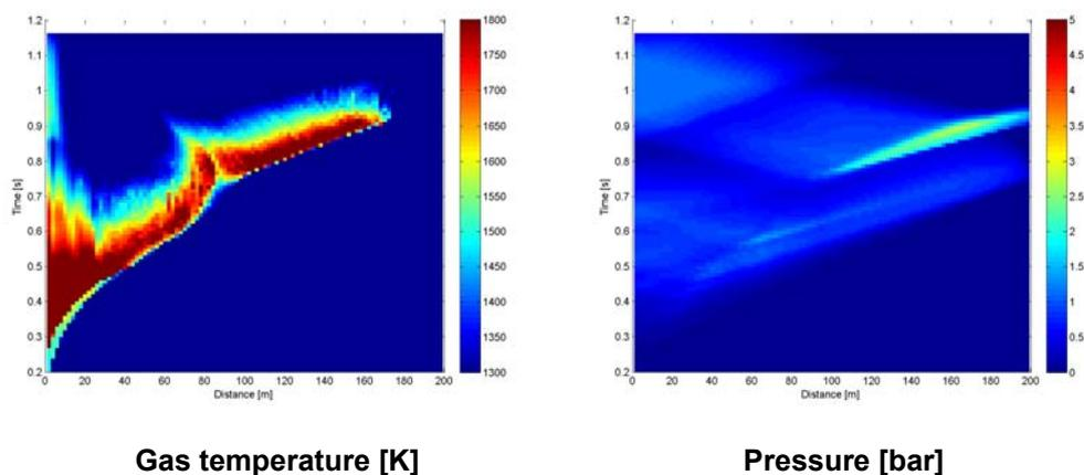
Figure 6 - Simulated 'Double Strong' explosion results
