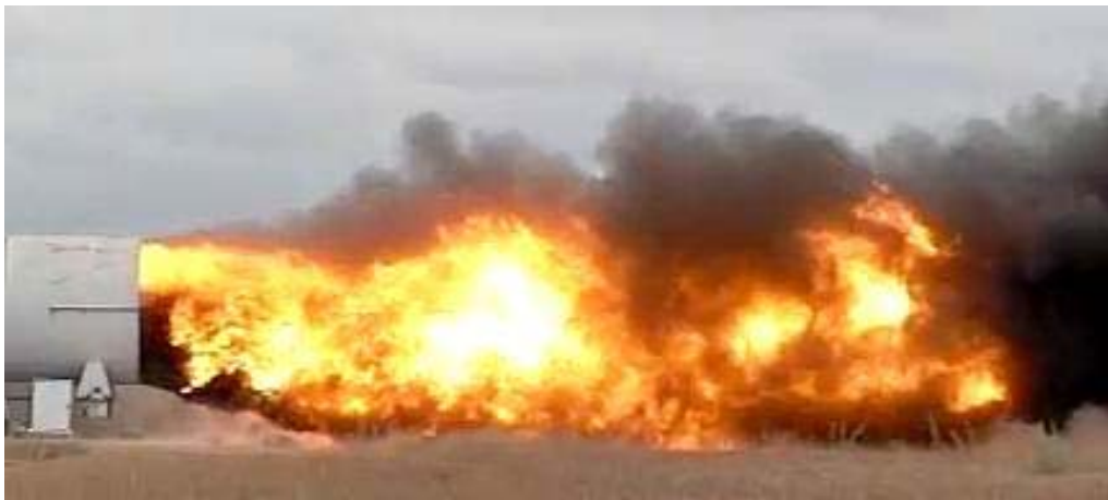
Figure 3 - Results of a 'Seminar' coal dust explosion at Kloppersbos
