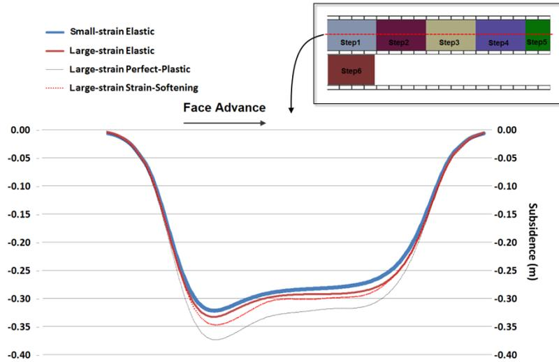
Figure 5 - Subsidence after completion of step 6
