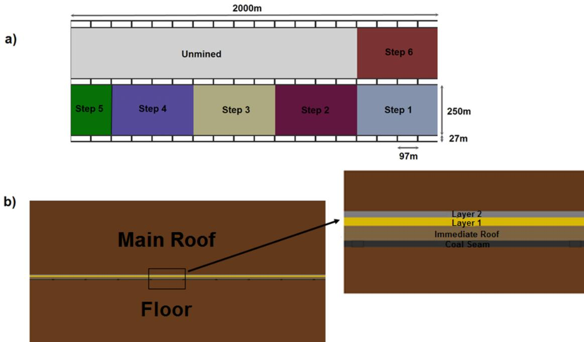
Figure 1 - Overall layout of the modelled longwall panel
