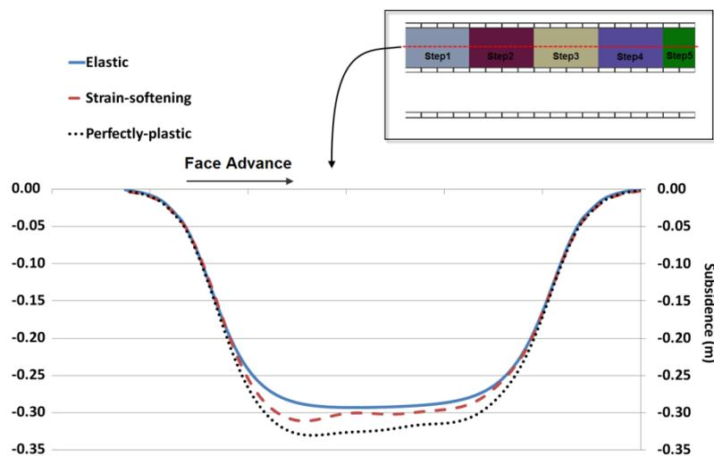
Figure 4 - Subsidence after completion of first panel (step 5)
