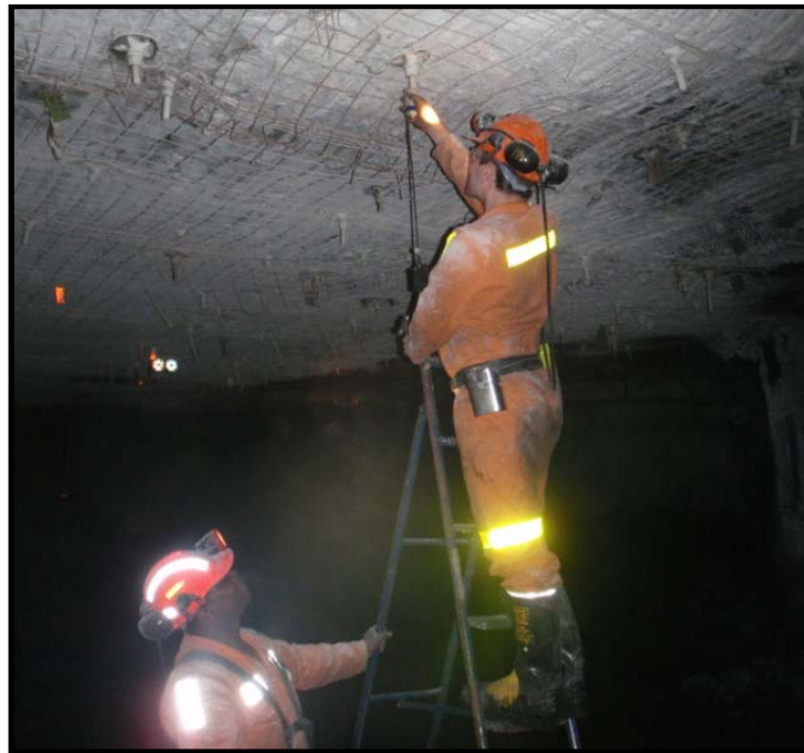
Figure 3 - Photo showing transducer (vertical) held at the end of bolt (i.e. collar of hole) at Manadalong Coal Mine
