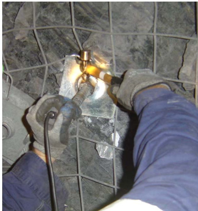
Figure 4 - Photo showing tapping device that is used to make contact with the nut of resin bolt
