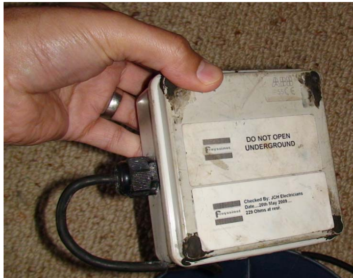
Figure 2 - Analogue/Digital Converter encased in closed unit for coal mine operations
