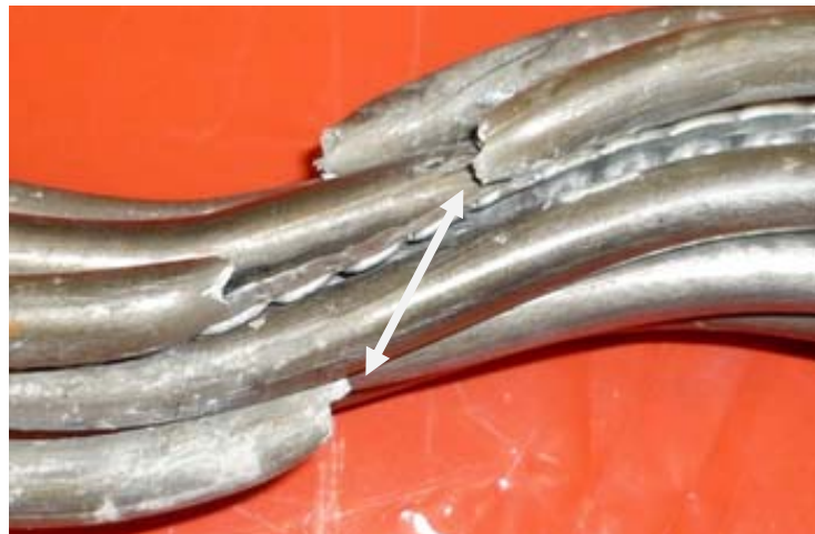
Figure 11 - Strand necking and flattened tube
