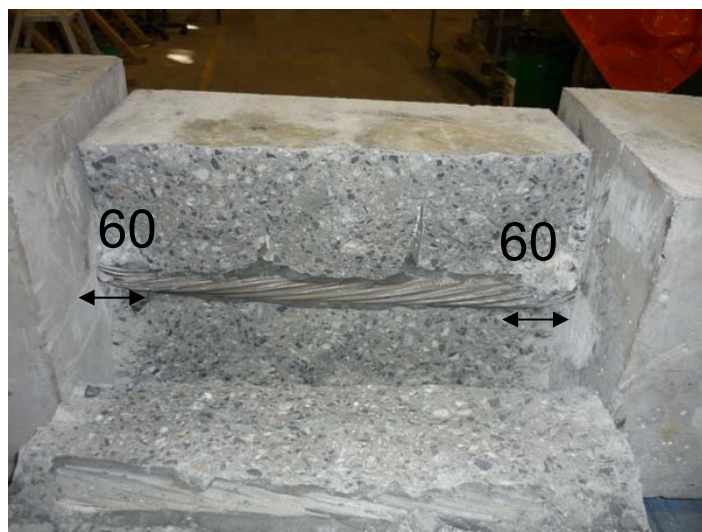
Figure 6 - Concrete / grout crushing and cable bolt deformation in the vicinity
