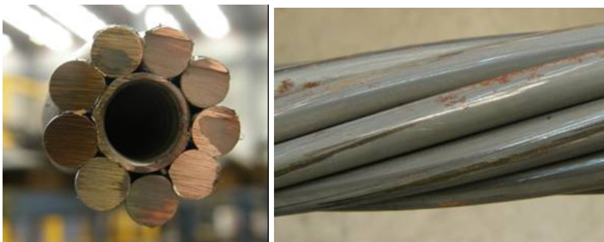
Figure 1 - Cross section and side view of nine strand TG cable bolt
