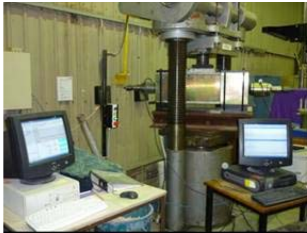
Figure 3 - Assembled double shear apparatus in 500 tonne testing machine
