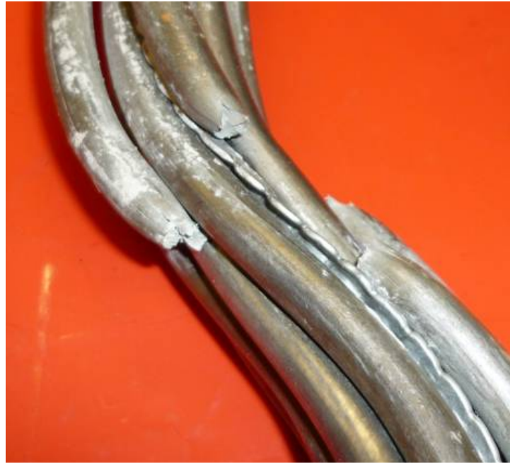
Figure 10 - Strand necking and flattened tube
