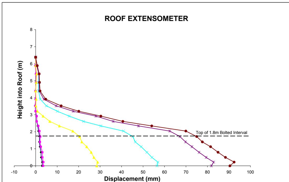
Figure 2 - Roof behaviour adjacent to longwall extraction
