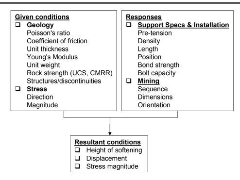
Figure 2 – Elements of uncertainties in roof support design
