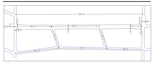
Figure 4 – LW 108 install road as mined dimensions (in meters)
