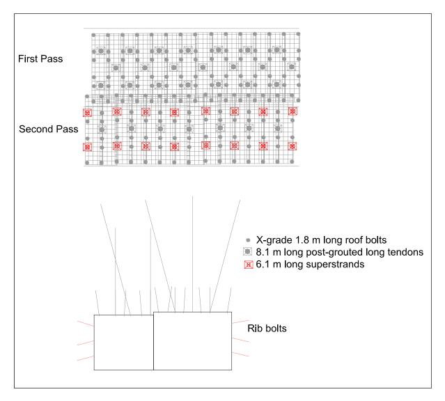
Figure 15 – Recommended roof support design
