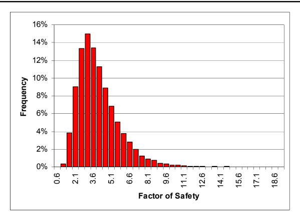
Figure 16 – Probability distribution of buckling failure mechanism (9.5 m wide areas)
