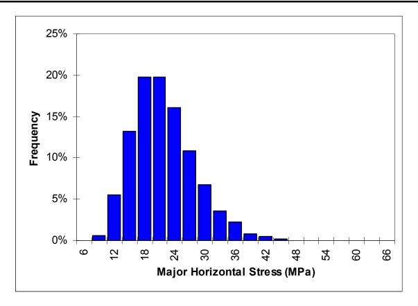
Figure 14 - Probability distribution of expected horizontal stress notching
