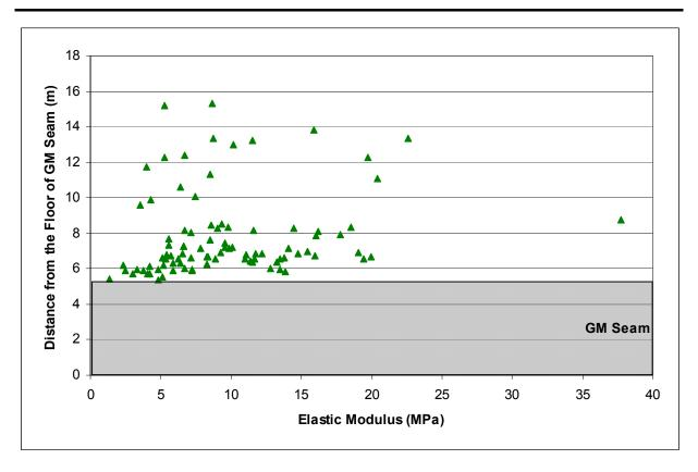
Figure 8 – Distribution of roof elastic modulus data with respect to the GM Seam
