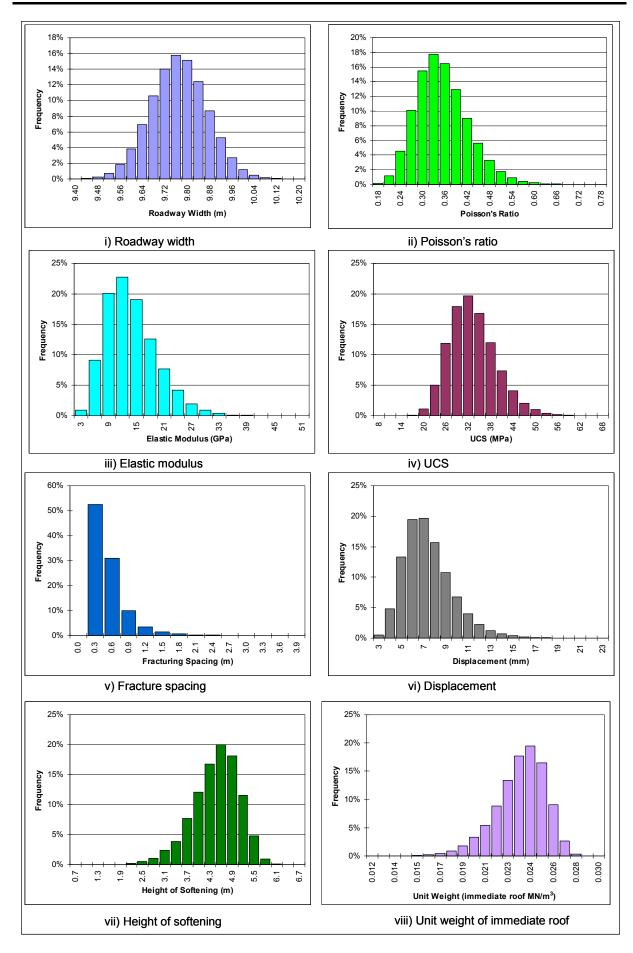
Figure 13 - Probability distributions of input parameters
