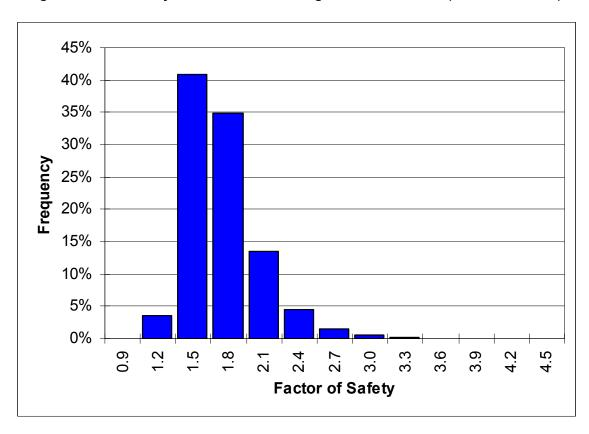
Figure 17 – Probability distribution of shear failure mechanism (9.5 m wide areas)
