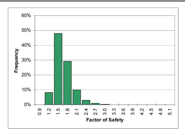
Figure 18 – Probability distribution of suspension long tendon failure (9.5 m wide areas)
