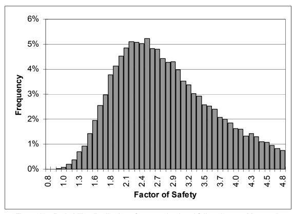
Figure 19 – Probability distribution of suspension bond failure (9.5 m wide areas)
