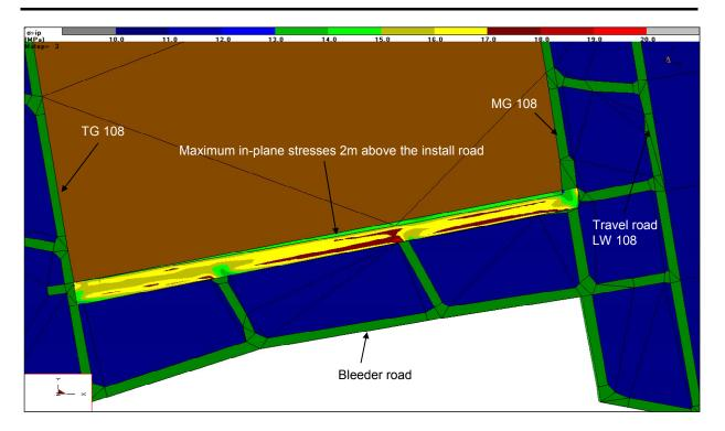
Figure 12 – Numerical modelling results (maximum in-plane stress) at the final stage (following the development and widening) of the install road
