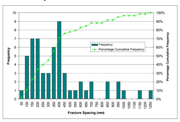
Figure 7 – Fracturing spacing distribution at long tendon anchorage horizon
