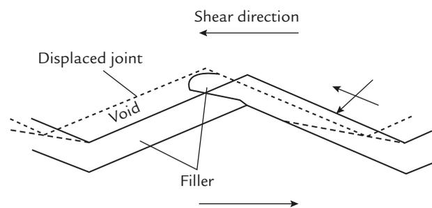
**Figure 2** Mechanism of infill failure for small thickness (modified from de Toledo & de Freitas, 1993).
