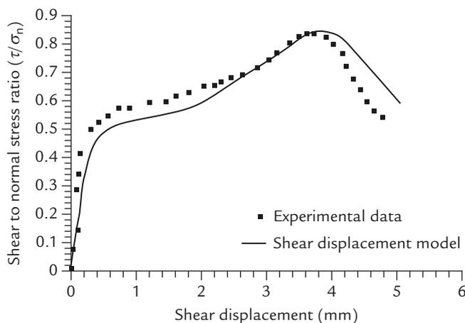
**Figure 3** Shear displacement criterion for soil-infilled joint.
