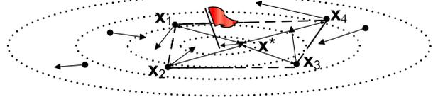
Fig. 1. Example of how the new particle  $\mathbf{x}^*$  is generated from  $\mathbf{x}_1, \mathbf{x}_2, \mathbf{x}_3$  and  $\mathbf{x}_4$  using the OD crossover operator. The flag indicates the optimum particle, and the arrow represents particle velocity.
