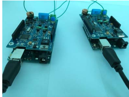
Figure 13: Two Mamba shields connected directly by two wires
