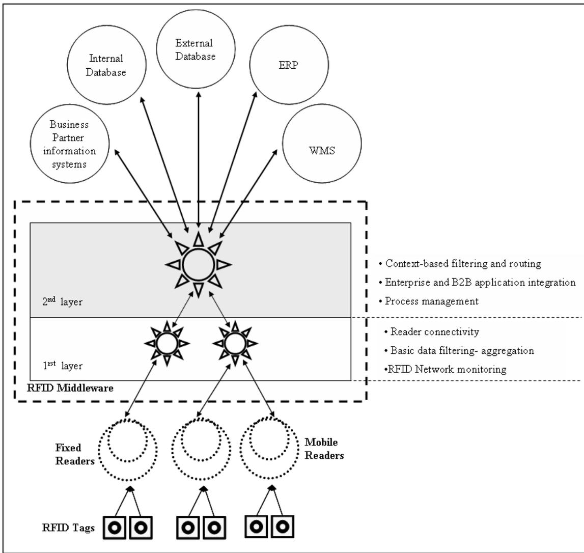
Figure 1: Positioning RFID middleware in an RFID system (www.forrester.com)
