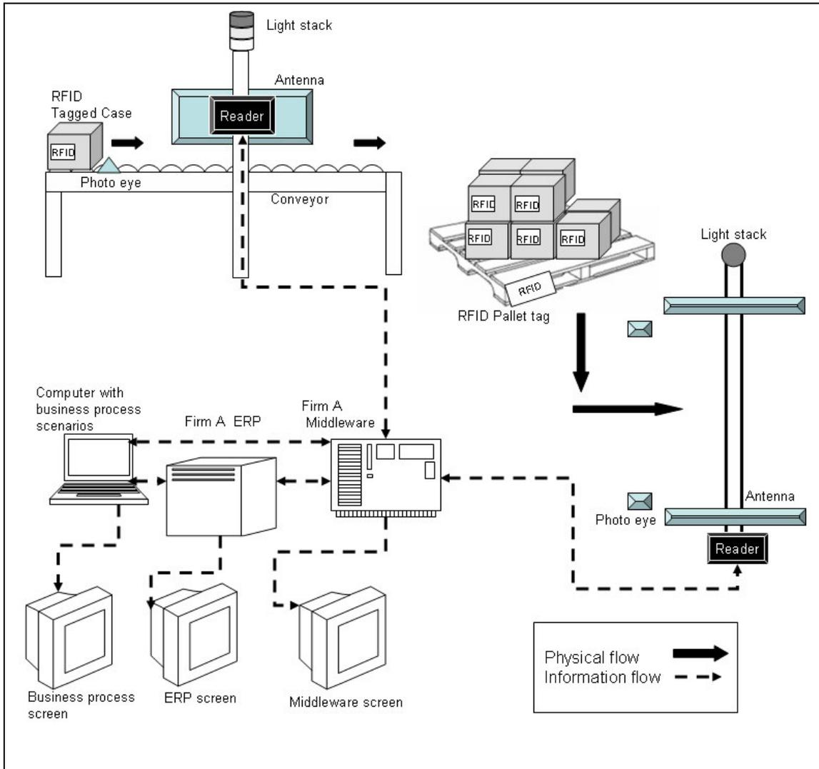
Figure 5: Technological infrastructure of the laboratory
