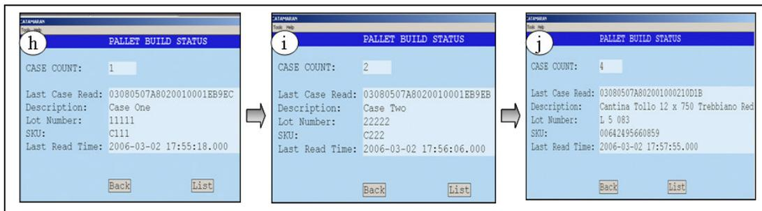
Figure 8: Automatic update of cases tags (c-Tag) in the palette and corresponding screen shots
