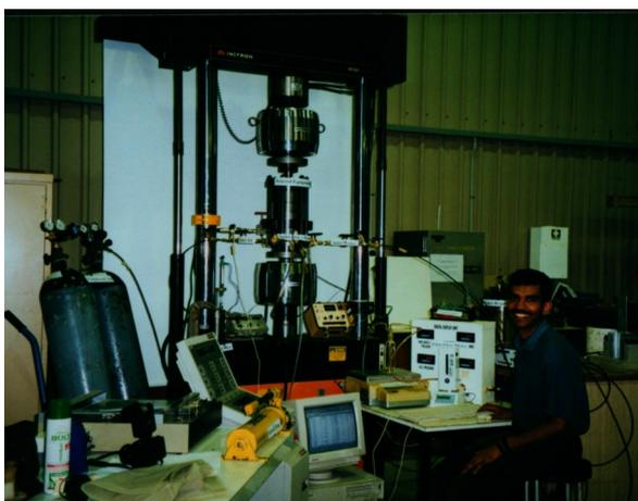
Figure 3: Experimental setup for Two-Phase, High pressure Triaxial Apparatus.
