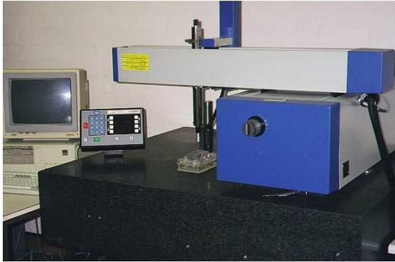
Figure 1: Mapping of joint profiles using the digital coordinate profiling apparatus
