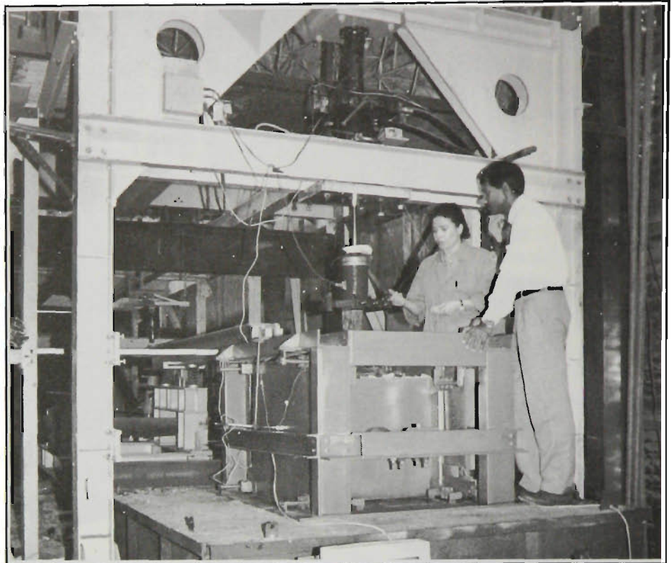
Ms Daniela Ionescu and Dr Buddhima Indraratna at work on sophisticated equipment designed at the University and constructed at the Railway Services Authority which can simulate the loads and displacements induced by the passage of trains on the railway track system
