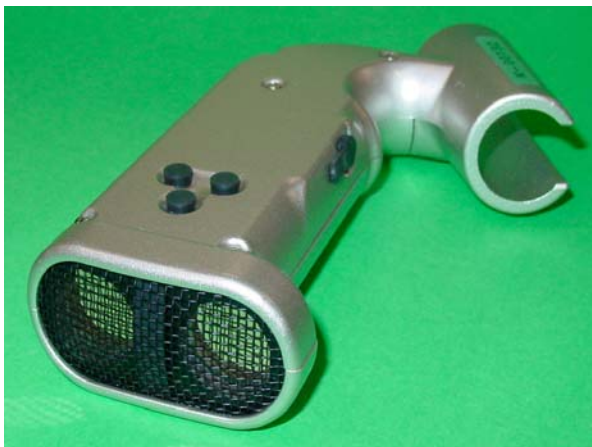
Fig. 1. K-Sonar ultrasonic sensor is designed with a mount point to fit on a blind person's cane.
