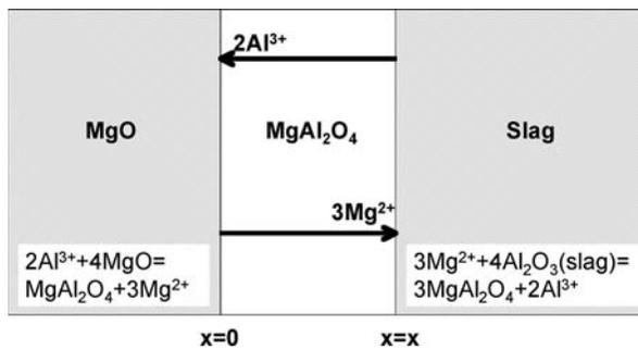
Fig. 5—Schematic showing the growth of a spinel ( $\text{MgAl}_2\text{O}_4$ ) on MgO.
