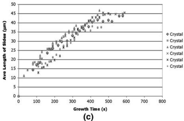
Fig. 4—Crystal size as a function of time at (a) 1420 °C, (b) 1440 °C, and (c) 1460 °C.
