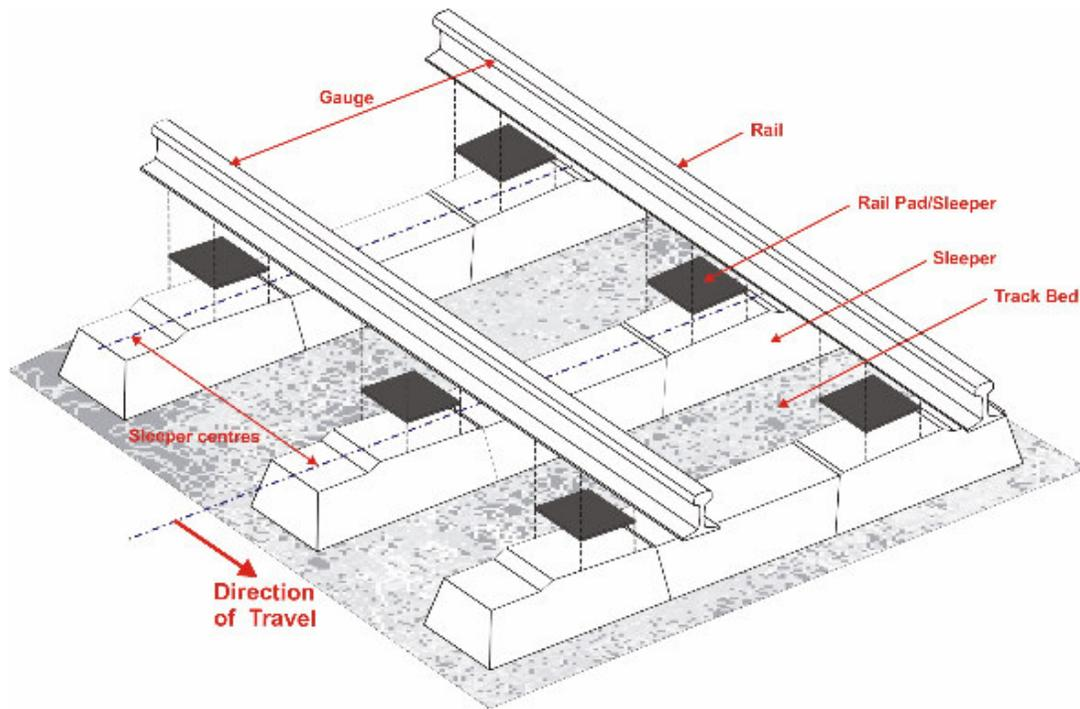
**Figure 1** Typical ballasted railway tracks from D-Track (Steffens, 2005)
