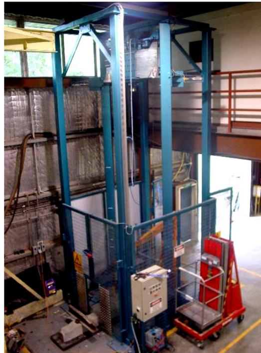
**Figure 4. High-capacity impact testing machine at University of Wollongong**
