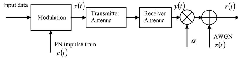
Fig. 1. Simplified UWB transmission model.
