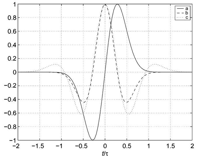
Fig. 3. (a) Transmitted Gaussian monocycle pulse  $w_t(t)$  with pulse width of  $2\tau$ . (b) Received pulse  $w_r(t)$  at output of receiver antenna. (c) Normalized autocorrelation coefficient  $\rho$  as a function of normalized time delay  $\Delta/\tau$ .
