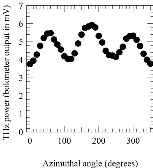
Fig. 2. Azimuthal-angle dependence of THz emission from sample.
