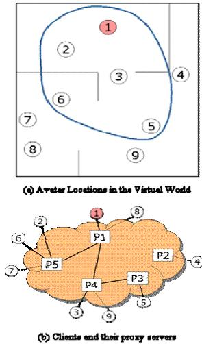
Figure 1. Distributed Proxy Architecture for Immersive Communications
