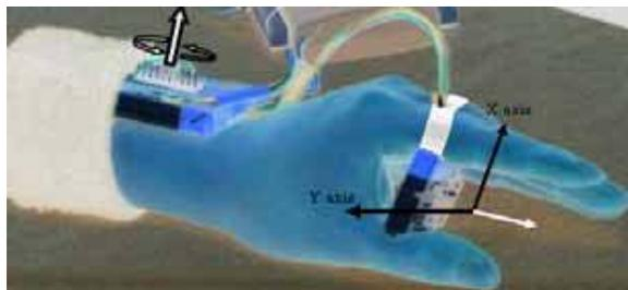
Figure 2 – Mounting of the sensors on hand
