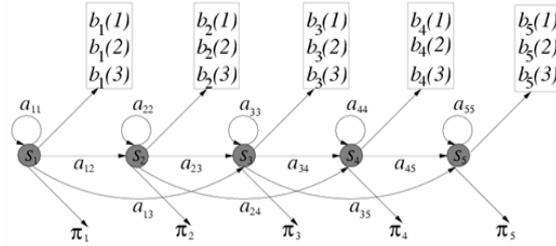
Figure 1 –The architecture of a typical Hidden Markov Model<sup>[12]</sup>
