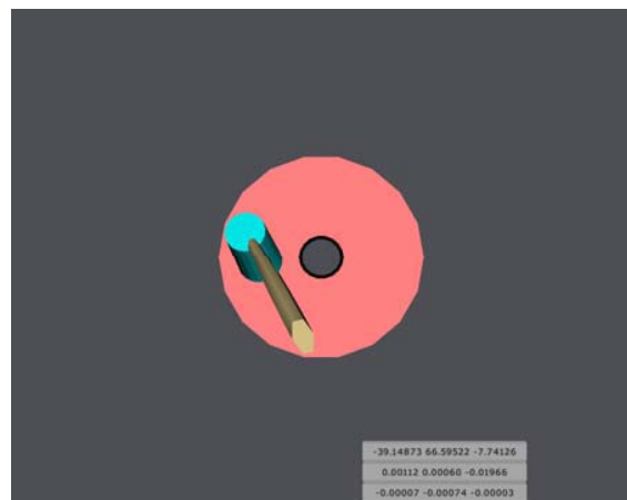
Fig. 1. 6DOF Peg-in-hole haptic virtual environment
