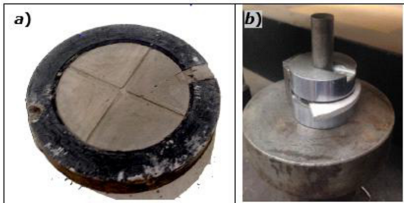
Fig. 3. a) Typical disc sample; b) Punch shear apparatus.
