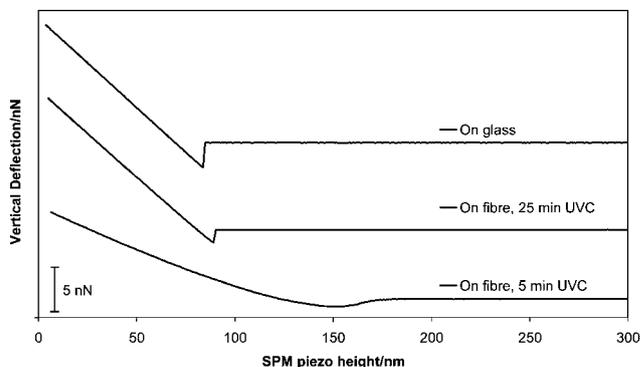
**Fig. 9** SPM approach indentation curves carried out in a pH 3 environment on different surfaces.
