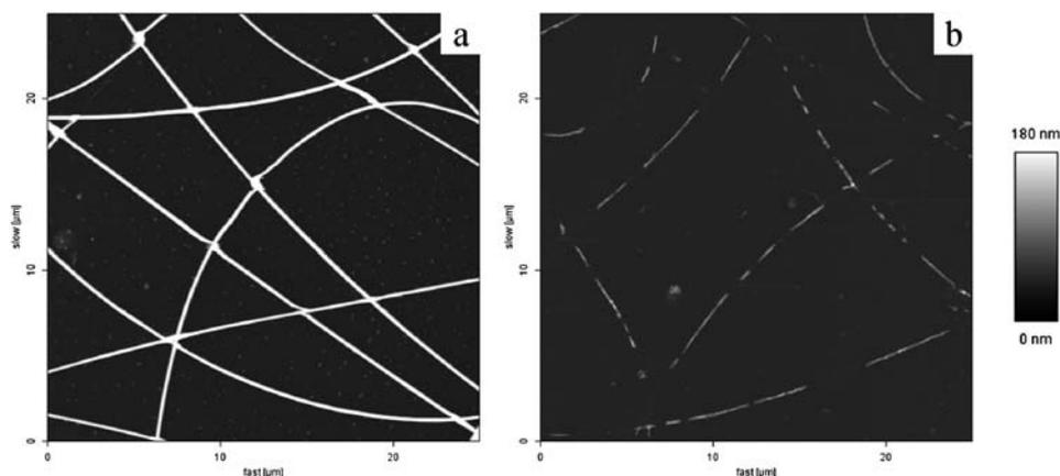
**Fig. 4** SPM height image of PAA fibres UVC treated for 25 min in a (a) nitrogen atmosphere and (b) in an air atmosphere.
