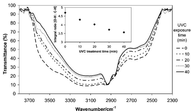
**Fig. 5** FTIR spectra of PAA with increasing UVC exposure time and inset showing the ratio of the integral intensity of the carboxylic acid O–H stretch ( $3700\text{--}2400\text{ cm}^{-1}$ ) to the alkane C–H stretch ( $3000\text{--}2850\text{ cm}^{-1}$ ).
