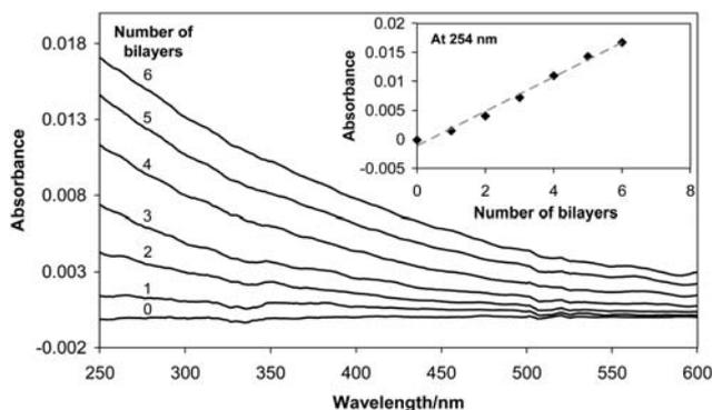
**Fig. 11** UV-Vis spectra of the PAA-PAH multilayer film increasing in absorbance with number of bilayers.
