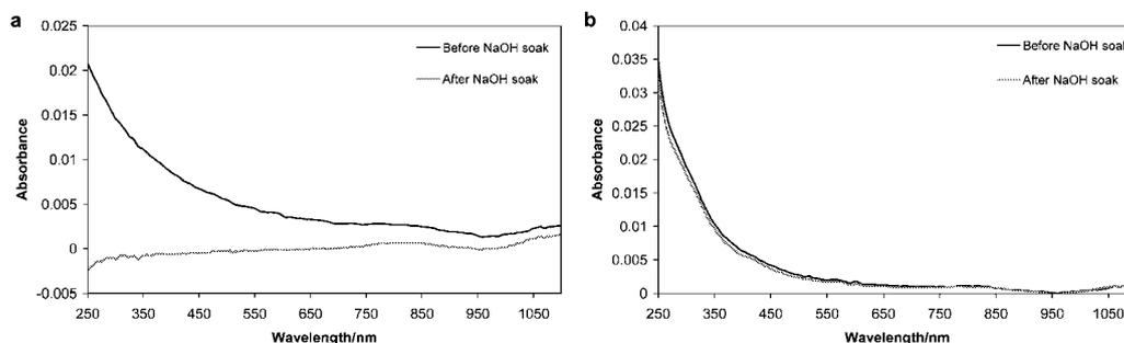
**Fig. 12** UV-Vis spectrum of a 6 bilayer PAA-PAH film on quartz before and after soaking in 0.1 M NaOH for 10 min (a) with no UVC exposure and (b) after 8 min of UVC exposure.
