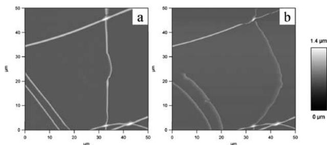
**Fig. 8** SPM height image of PAA nanofibres irradiated by UVC for 5 min and then immersed in a pH 3 electrolyte on (a) the first scan showing a mostly stationary fibre from top to bottom and (b) the fourth scan showing the same fibre being snagged and dragged whilst anchored at the two crossover points.
