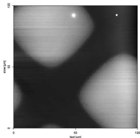
**Fig. 10** SPM height image of a dry, thin PAA film, UVC treated while masked with a TEM grid then soaked in acidic solution to remove uncrosslinked PAA, revealing the pattern of the mask.
