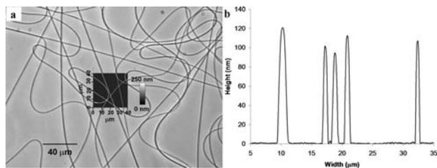
**Fig. 2** (a) Optical image of dry electrospun PAA fibres with SPM image overlaid in the centre and (b) representative single scan taken from the SPM image showing cross-sections of 5 fibres.
