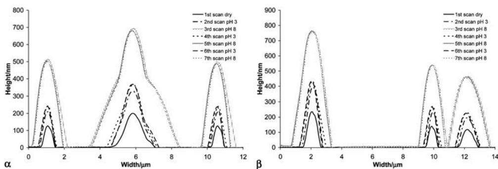
**Fig. 6** Representative traces taken from consecutive SPM images in different environments. These traces were taken from the positions shown by the dashed lines ( $\alpha$  and  $\beta$ ) in Fig. 1 for PAA nanofibres exposed to UVC radiation for 5 min in air.
