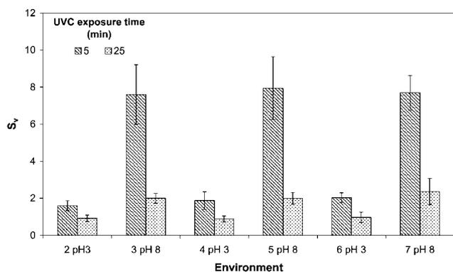
**Fig. 7**  $S_s$  over traces taken from three samples at both 5 and 25 min UVC treatment time and after successive changes in solution pH. Error bars indicate one standard deviation in swelling ratio.
