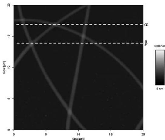
**Fig. 1** Typical SPM image of dry PAA nanofibres. Traces taken at the dashed lines labelled ‘ $\alpha$ ’ and ‘ $\beta$ ’ were used to calculate the volume change of the fibres over consecutive images.
