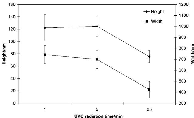
**Fig. 3** Dry fibre height and width averaged over points taken from triplicate samples at 1, 5 and 25 min UVC radiation time in an air atmosphere with error bars indicating one standard deviation. These fibres were imaged dry after UVC irradiation.
