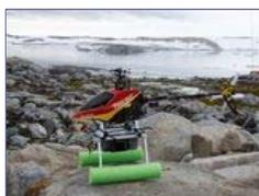
The first UAV, based on a remote controlled helicopter with a camera, at Robinson Ridge in 2010.
