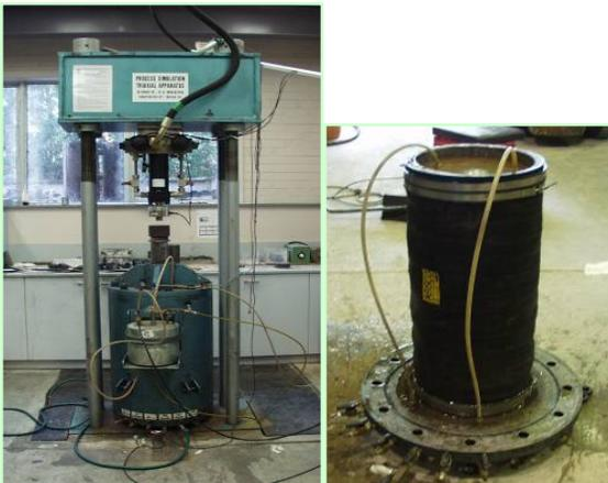
Figure 27: (a) Large-scale triaxial rig, (b) soil specimen
