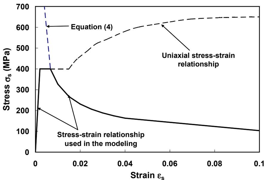
Figure 2. Stress-strain relationship of longitudinal bar
