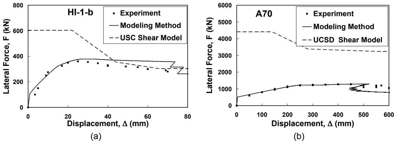
Figure 3. Experimental results compared with analytical predictions
