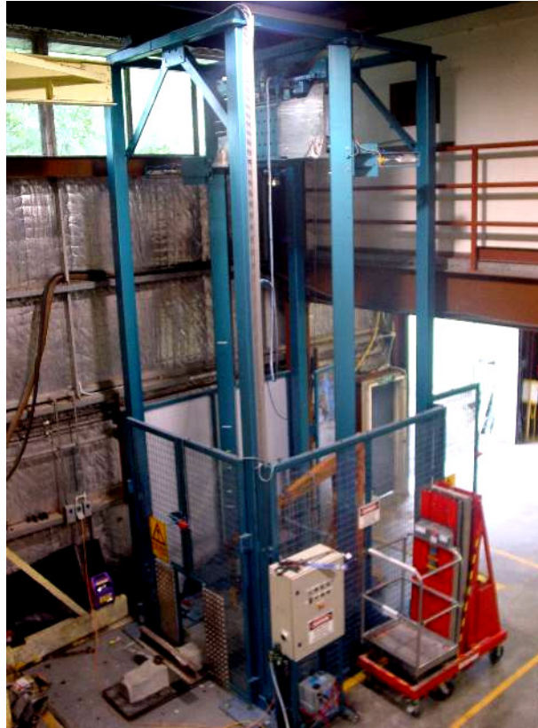
Figure 2 High-capacity drop-weight impact machine at the University of Wollongong
