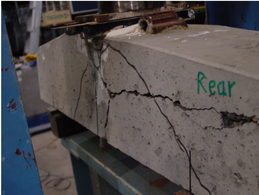
Figure 8. Behavior of test concrete sleeper under ultimate impact load.
