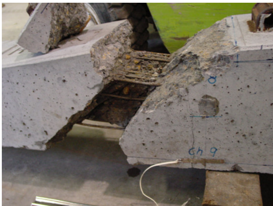
Figure 7. Behavior of test concrete sleeper under static load.
