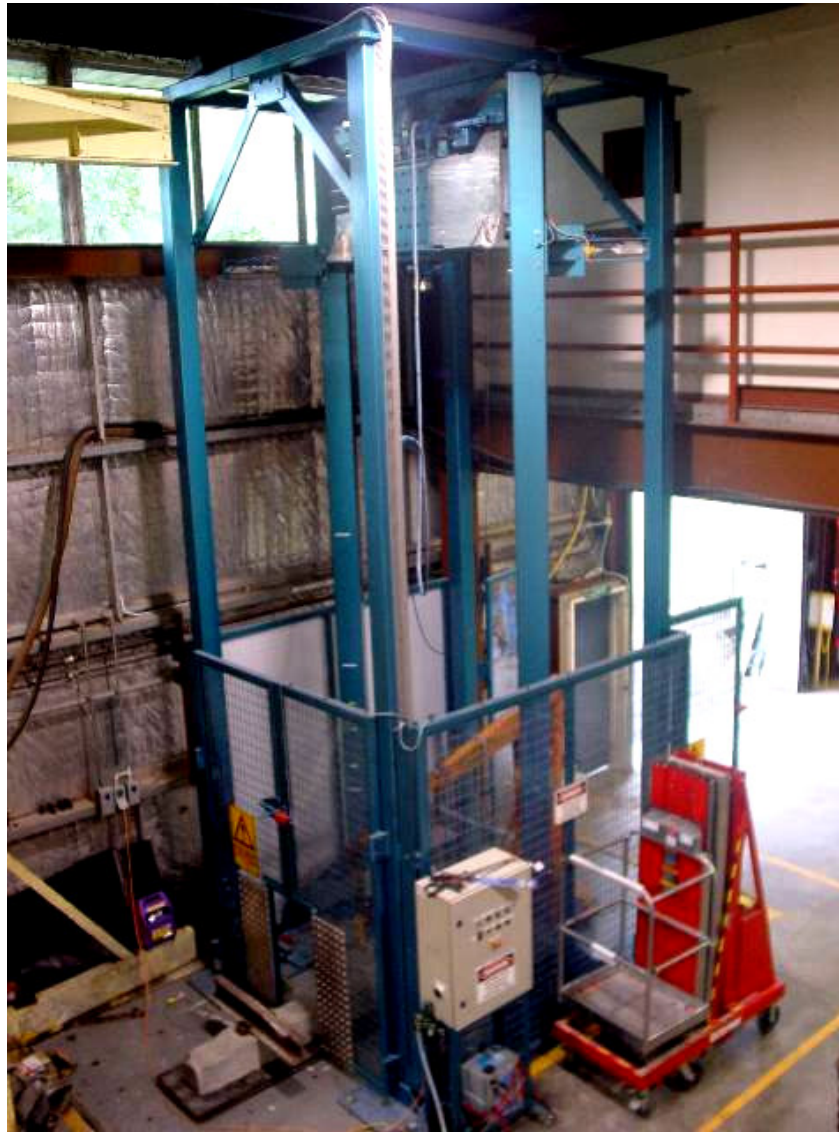
Figure 3 New high-capacity drop-weight impact testing machine at the University of Wollongong
