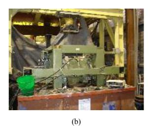
Figure 4 Large-scale triaxial apparatus built at the University of Wollongong, (a) large-scale triaxial apparatus and (b) Large prismoidal triaxial apparatus (Indraratna et al. 1998) The model parameters  $\beta$ ,  $\chi$  and  $\mu$  can be determined using the breakage measurements and other experimental results, as shown in Fig. 5.
