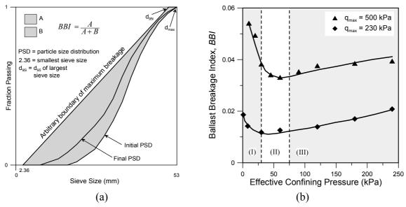
Figure 2 (a) Evaluation of the Ballast Breakage Index *BBI* (b) Effect of confining pressure on ballast degradation under cyclic loading (Indraratna et al. 2005)
