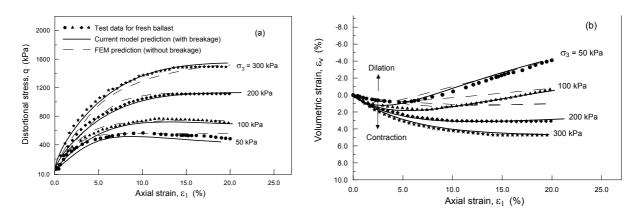
Figure 6 Experimental data of ballast compared with FEM analysis results and analytical model predictions, (a) stress-strain, and (b) volume change behaviour (Indraratna and Salim, 2005)
