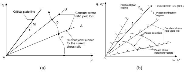
Figure 3 (a) Yield loci represented by constant stress ratio lines in *p-q* plane and (b) Plastic strain increment vectors and plastic potentials (Salim and Indraratna, 2004, Indraratna and Salim, 2005)
