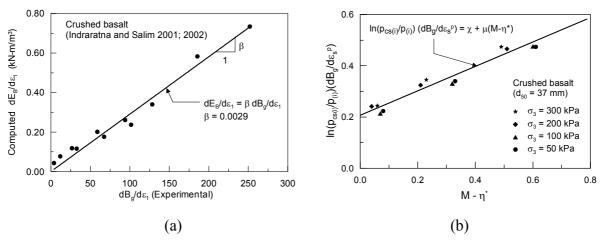
Figure 5 (a) Relationship between the rate of energy consumption and rate of particle breakage and (b) Modeling of rate of particle breakage during triaxial shearing (Salim and Indraratna, 2004, Indraratna and Salim, 2005)
