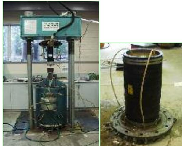
Figure 30 (a) Large-scale triaxial rig, (b) soil specimen
