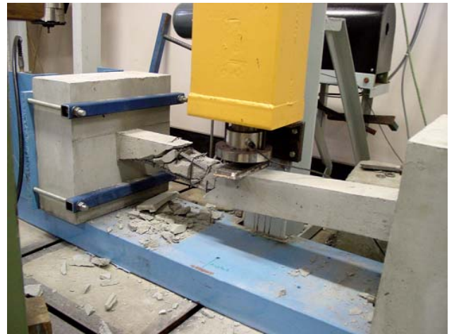
Figure 8. Impact failure of rebar type specimen.
