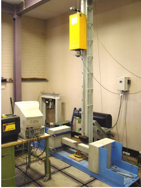
Figure 3. Impact testing setup
