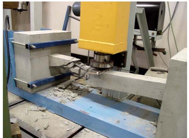
Figure 8. Impact failure of rebar type specimen.
