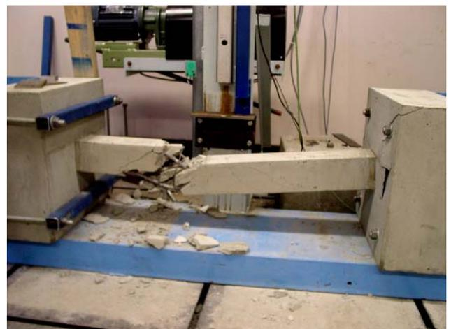
Figure 9. Impact failure of ribbed wire type specimen.
