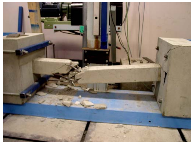
Figure 9. Impact failure of ribbed wire type specimen.
