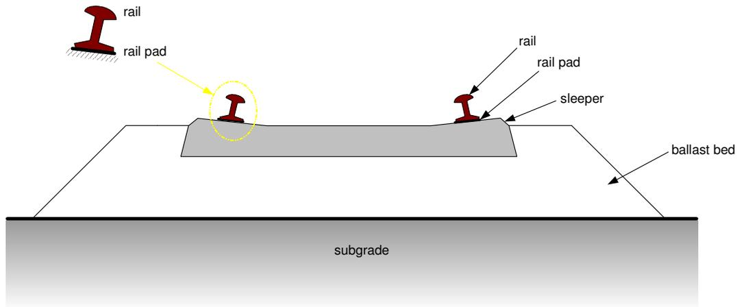
**Figure 3.** Typical ballasted railway track (Remennikov and Kaewunruen, 2005)
