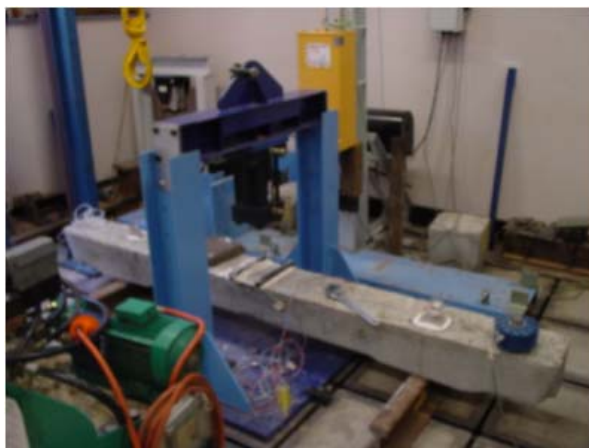
Figure 5. Hogging moment test
