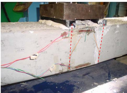
**Figure 8:** Initial cracks
