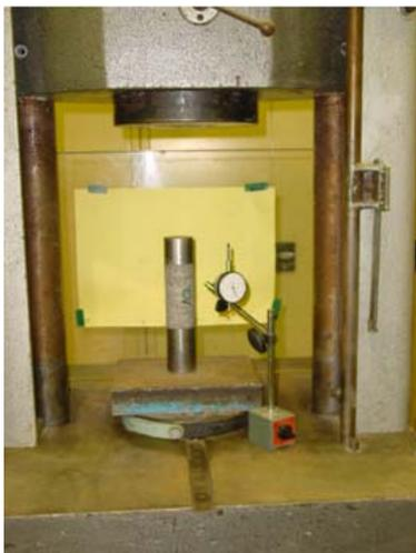
**Figure 4.** Uni-axial testing
