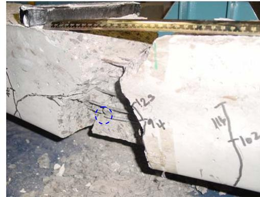
**Figure 10:** Prestressing wire damages
