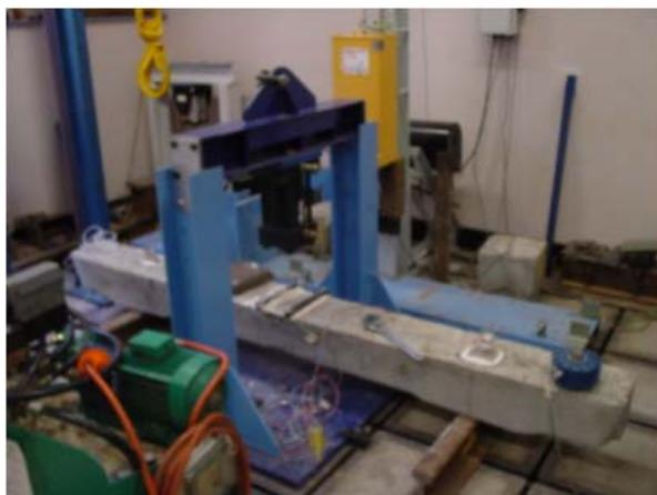
**Figure 5.** Hogging moment test
