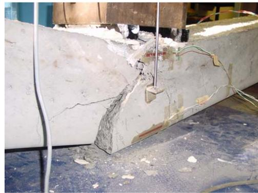
**Figure 9:** Concrete crushing
