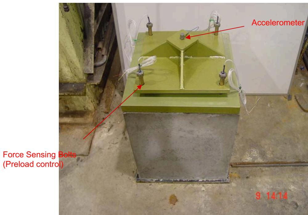
**Figure 4: Detailed View of Rail Pad Tester**
