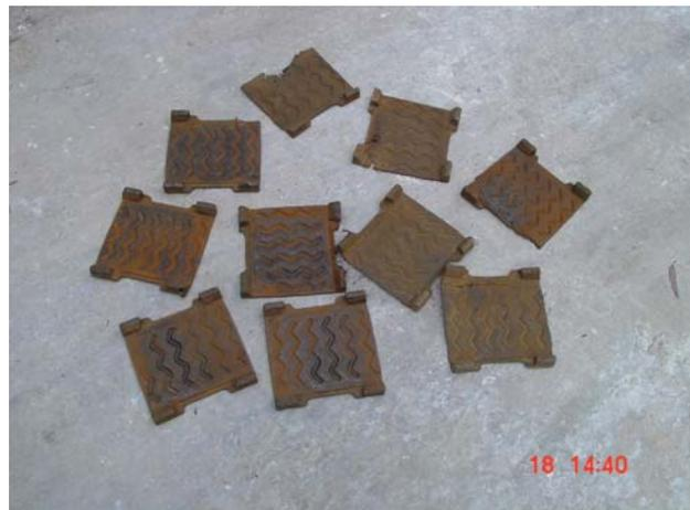
**a) after 99 MGT in service on RailCorp track**
