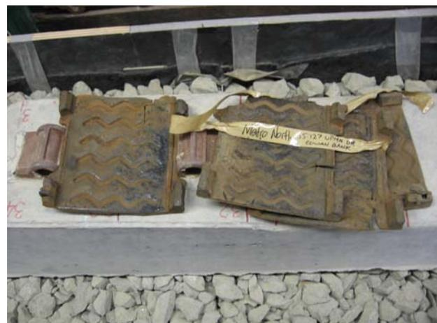
**b) after 110 MGT in service on RailCorp track**
