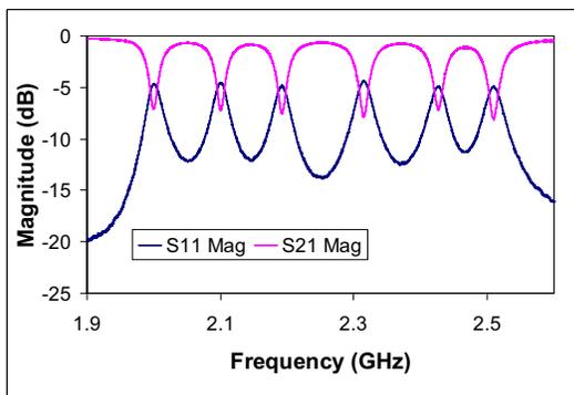
Fig. 18. Measured S-parameters of the manufactured multiresonator.
