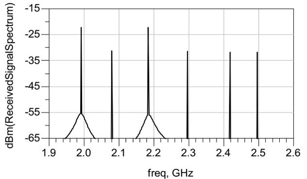
Fig. 12. Received signal from chipless transponder with ID 101000.
