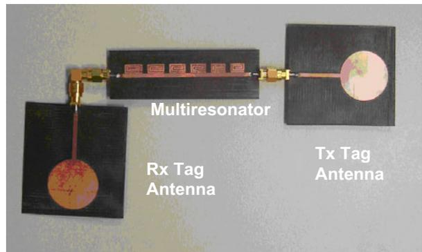
Fig. 27. Photograph of prototype chipless RFID Tag
