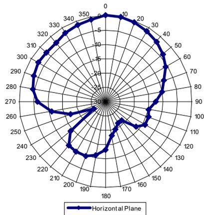
Fig. 23. Reader antenna radiation patten – horizontal plane.
