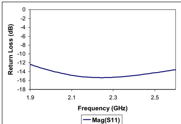
Fig. 5. Simulated return loss of the UWB tag antenna
