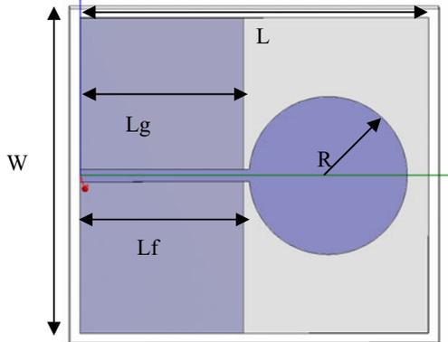
Fig. 4. UWB Monopole Antenna for chipless RFID tag
