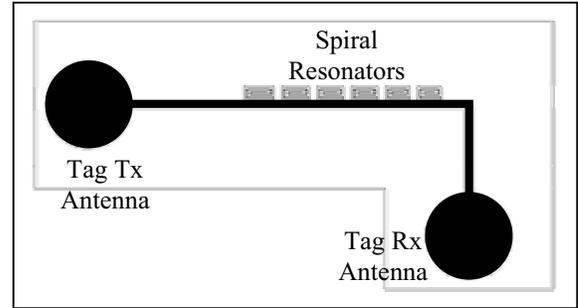
Fig. 2. Layout of the chipless RFID transponder.
