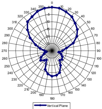
Fig. 24. Reader antenna radiation patten – vertical plane.
