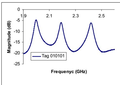
Fig. 19. Measured S11 of multiresonator with spectral signature "010101".
