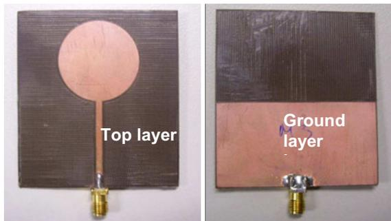
Fig. 13. Photograph of the manufactured UWB monopole
