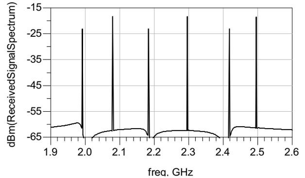
Fig. 11. Received signal from chipless transponder with ID 010101.
