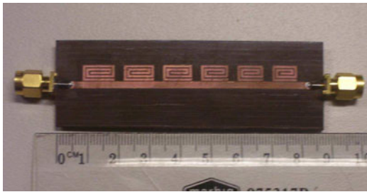
Fig. 17. Photograph of the manufactured multiresonator with spiral resonators.
